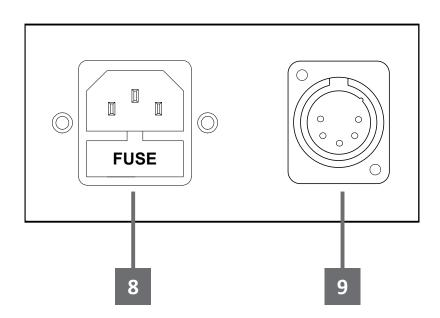
8 AC MAINS INPUT 9 POWER SUPPLY OUTPUT
